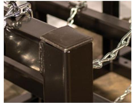
All barricade rack end tops are capped with high-density polyethylene caps to reduce injuries from sharp edges while preventing dirt build-up and corrosion inside tube for a clean, quality look.
