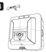
Secure the unit with the  $\#4-40 \times 3/8$ " screw and snap the nameplate over the screw.
