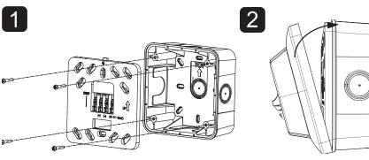
Attach the mounting plate to the mounting box with the 4 screws.
