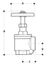
A= 3.9" (98.5mm) B= 8.3" (OPEN) (211mm) B= 7.2" (CLOSED) ((183.1mm) C= 2.0" (52mm) D= 2.0" (51.8mm)
